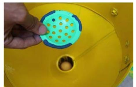
12. Place Strainer on the drain mouth of the Funnel and press down to let M-Seal spread and fix the Strainer.
