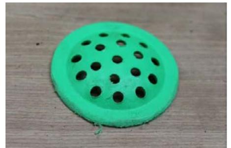
11. Place strips of M-Seal on the strainer, curved along its edges as shown here.
